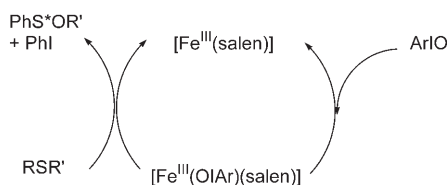
Scheme 2. Proposed catalytic cycle for iron-catalyzed asymmetric oxidation of sulfides.
